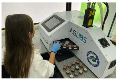
Agrorobotica's machine uses laser pulses to measure within minutes how much carbon dioxide the soil contains.
